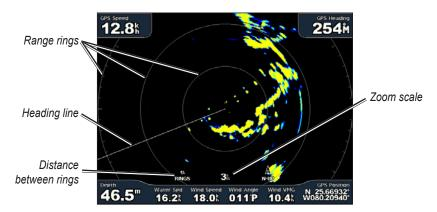
The zoom scale represents the distance from your position (the center) to the outermost ring. Each ring represents an even division of the zoom scale. For example, if the zoom scale is set at three kilometers, each ring represents one kilometer from the center out. Use the **RANGE** (+/-) keys (GPSMAP 4000 series) or the series and keys (GPSMAP 5000 series) to adjust the zoom scale.
